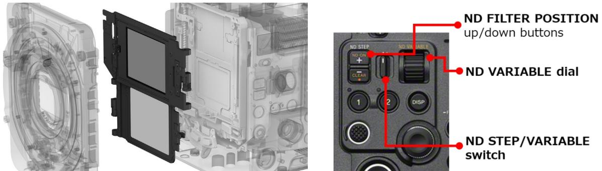
With physical ND filters no longer needed, operators can adjust the electronic filter density by simply rotating the ND dial. Operators can maintain a constant depth of field by adjusting the electronic ND filter and the iris control together.
